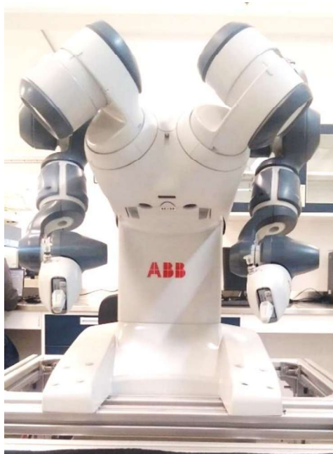
Figura 1. Robot ABB YuMi IRB 14000.
